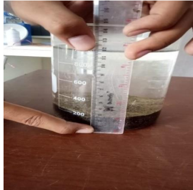
Gambar 4. 22 Pengujian Kadar Lumpur
